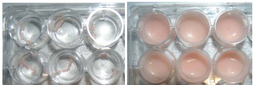
10 mg hotdog samples in 100 microliters of water, before and after 60 seconds of homogenization.
