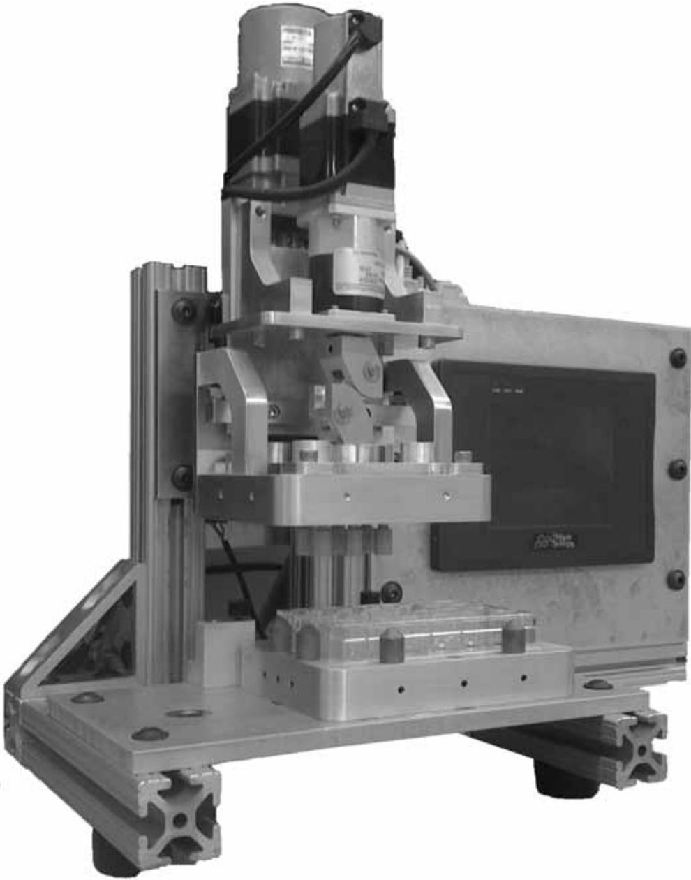
CMI's prototype tissue homogenization instrument
