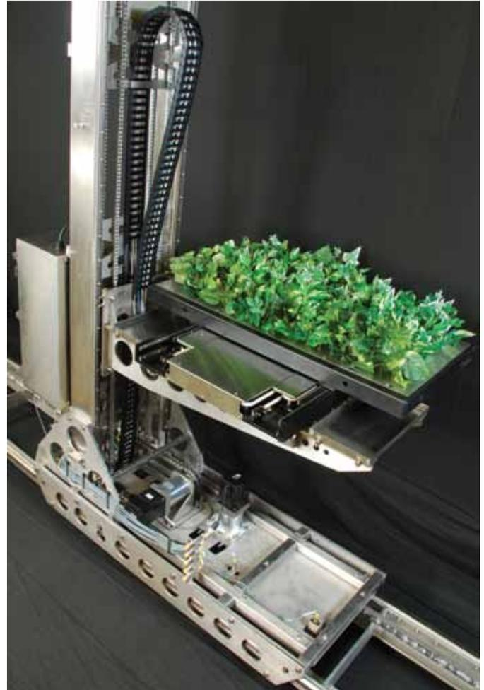
Custom-made robot being tested
