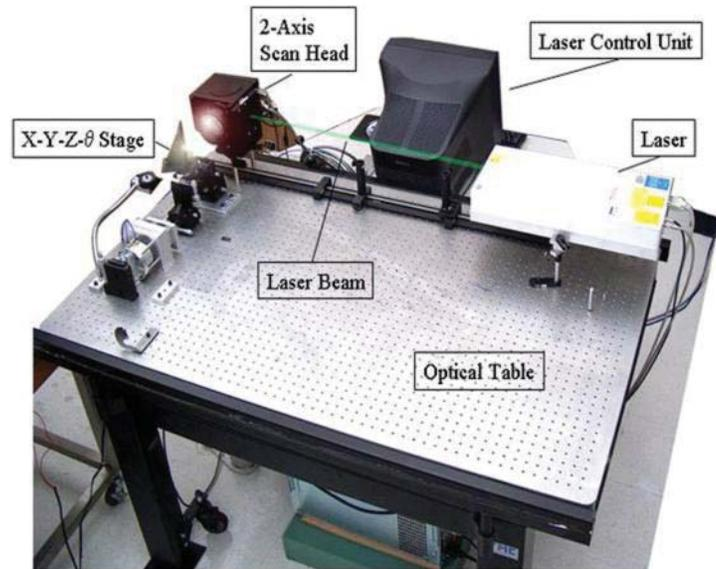
The experimental apparatus is comprised of a pulsed Nd:YAG laser (emitting at 355nm) directed through a 2-axis Scan Head. Since the pulsed UV laser is not easily visible, an auxiliary red alignment laser was used for multilevel alignment. Since light rays can be converged to a focal point, the distribution of laser intensity as a function of focal depth can be selectively exposed by varying laser doses from Gaussian-like spot.
